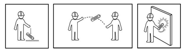
The zero-g safety function can prevent the uncontrolled output of commands in specific emergencies. The G sensor can detect if the transmitter receives a hard impact, dropped or thrown. These features can deactivate either the complete radio system or only the safety-relevant function relays. Alternately, a pre-defined output (e.g. crane horn) can be triggered. Please contact your dealer for special settings.
