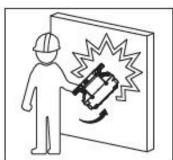
The zero-g safety function can prevent the uncontrolled output of commands in specific emergencies. The G sensor can detect if the transmitter receives a hard impact, dropped or thrown. These features can deactivate either the complete radio system or only the safety-relevant function relays. Alternatively, a pre-defined output (e.g. crane horn) can be triggered. Please contact your dealer for special settings.
