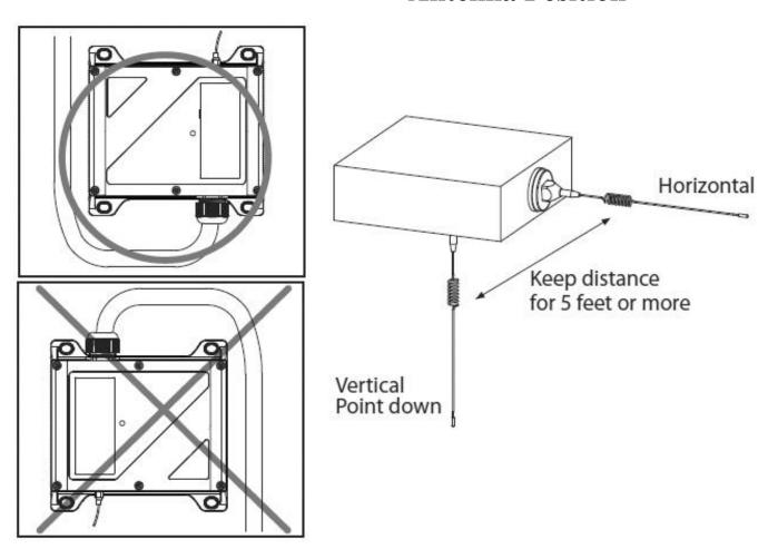
Mount Enclosure in the orientation shown above. Do not mount upside down. The Receiver Enclosure should be mounted in an area clear of large metal objects, away from crane electricification and with ideally unobstructed line-of-sight to the operator's area.
